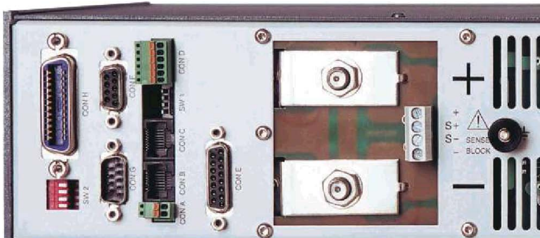
fig. 3 - 9 location of output terminals and analog programming connector on the rear panel (unit with optional PSC488)
