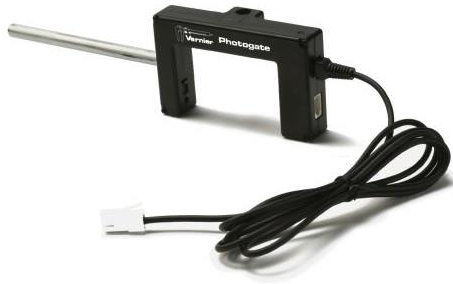
Figur 28: Photo Gate VPG-BTD
